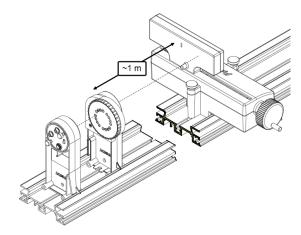
Figure 2. Setup with the Wireless Diffraction Scanner.
