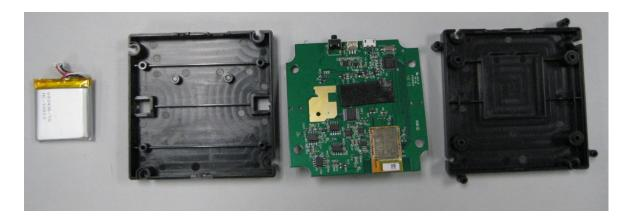
**Step 4:** Plug the replacement battery into the battery connector on the PC Board and carefully locate the battery into the bottom cover battery compartment as shown below. Lower the PCB into place.
