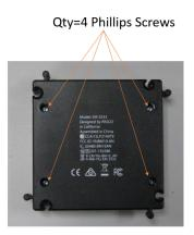
**Step 2:** Remove the bottom cover exposing the PC Board Assembly as shown below.
