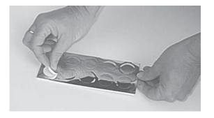
2. Carefully remove the protective backing paper.
