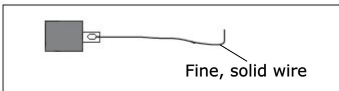
Figure 4. Wire attached to mass. Use to calibrate the Vertical Accelerometer.
