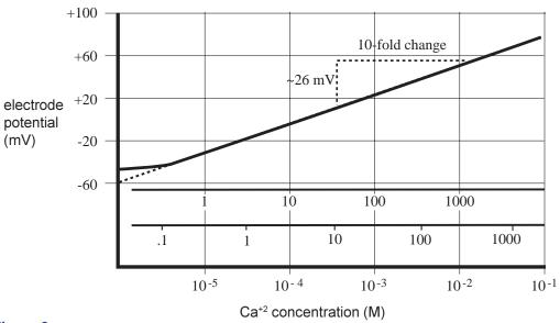
**Figure 3** Typical calcium electrode calibration curve
