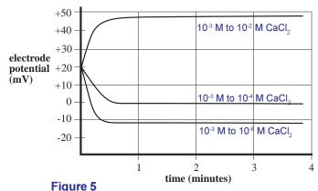
Typical electrode time response to step changes in CaCl
