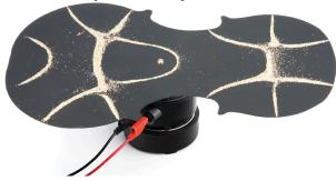
NOTE: The Chladni Violin Plate can also be used with the Mechanical Wave Driver (SF-9324). A banana plug is included with the Chladni Violin Plate as legacy support for connecting the plate to the Mechanical Wave Driver. However, the Wave Driver (WA-9855) is strongly recommended for experiments with the Chladni Violin Plate.
