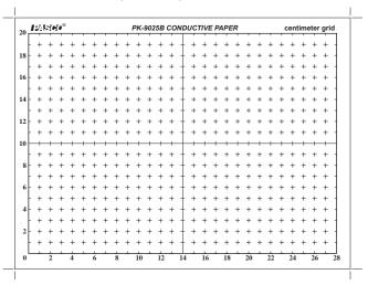
The pattern on the back of this page can be used to make photocopies of the conductive paper's grid pattern. Care has been taken to ensure that the size and location of lines and crossing points are the same as the pattern on the conductive paper. Students can draw the shape and size of their conductive ink electrodes on their copy of the grid paper. Once the sketch is drawn, students can transfer their readings of voltage or pattern of equipotential lines onto the sketch.
