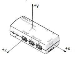
When motionless, the accelerometer measures +9.8 m/s<sup>2</sup> when pointing *away* from the ground and -9.8 m/s<sup>2</sup> when pointing *towards* the ground. This is useful for determining the //control.Node's orientation. For example, if the y-axis is pointing away from the ground, the **Acceleration - y** measurement reads 9.8 m/s<sup>2</sup> and the other axes measure 0.
