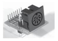
Digital Adapter (CI-6719) - enables the use of one or two ScienceWorkshop digital sensors with ELVIS.
