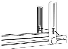
bumper protects the sensor from being hit by a cart.
