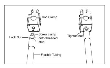
**6.** To attach the included three-finger clamp, first attach a rod clamp or double clamp to the flexible tubing. Mount the three-finger clamp in the rod clamp and tighten the thumbscrew to hold it in place.
