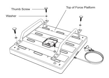
Handle installation on top of Force Platform
