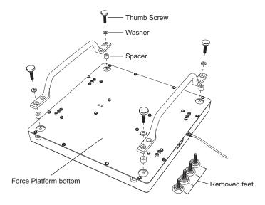
Handle installation on bottom of Force Platform
