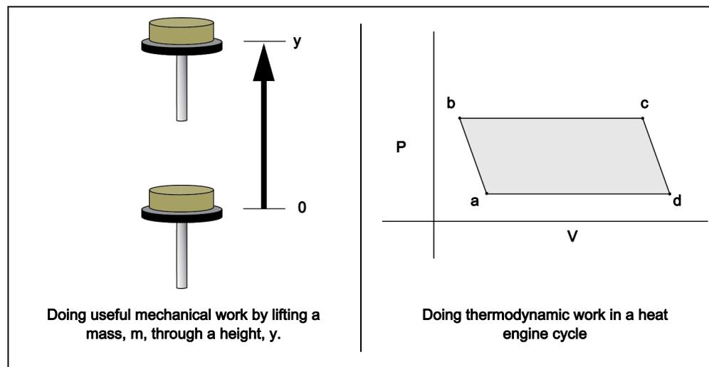
The PASCO Heat Engine/Gas Law Apparatus consists of a hollow cylinder with a low friction graphite piston that can move along the axis of the cylinder. The piston has a platform attached to it for lifting a mass. A metal can
