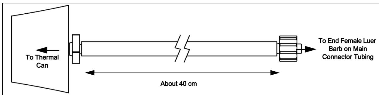
PASPORT Pressure Sensor Adapter Tubing: The male Luer barb on one end of the tubing connects to the side female Luer barb on the Main Connector Tubing. The quick-release connector on the other end of the tubing connects to a quick-release connector port on a PASPORT pressure sensor.
