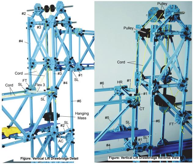
(\*Do not overtighten the Sliding Connectors that grasp the vertical #6 Beams. The middle section must be able to slide up and down the #6 Beam.)
