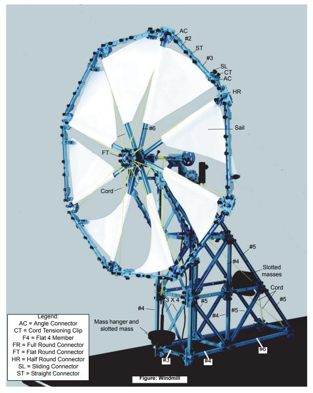
A template for the paper sails is included at the end of the instructions. Copy (or trace) the template and cut out the sail from a sheet of 8.5 by 11 inch (21.5 by 28 cm) paper.
