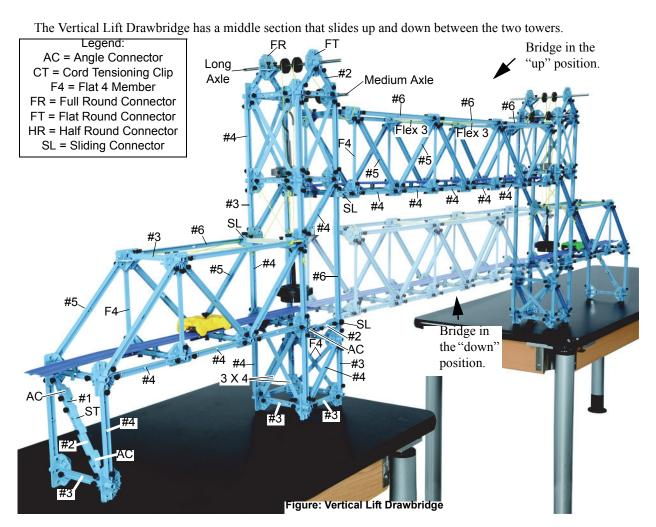
The middle section is counterbalanced by hanging masses connected by cords over pulleys. The hanging masses move up and down inside each tower.
