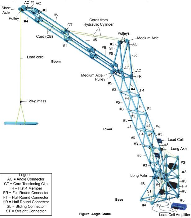
Use two #3 Beams and a Straight Connector to make ten extra #5 Beams for the Base and Tower. The hook on the end of the cord is a 20 g mass from the Hooked Mass Set (SE-8759). Slotted masses on the back of the base are counterweights for the Tower and Boom, and forces in the Tower and Base are measured by 100 N Load Cells connected to a Load Cell Amplifier. The Base width is a #4 Beam, the Tower width is a #3 Beam, and the Boom width is a #1 Beam.
