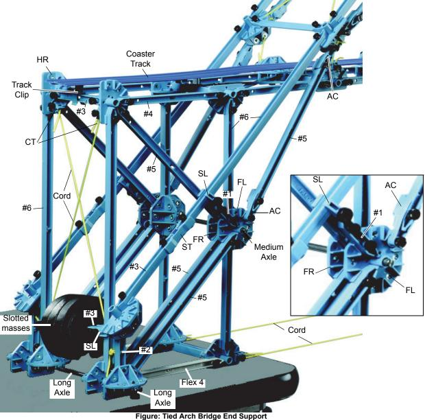
Use cord and Cord Tensioning Clips to cross brace the back of the end support. Tie cords between the bottoms of the two end supports.
