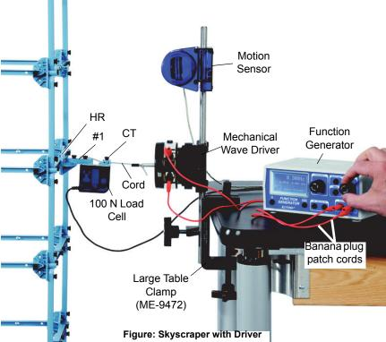
For example, replace a Straight Connector with a Half Round Connector. Add a #1 Beam to the Half Round. Attach a 100 N Load Cell (PS-2200) to the #1 Beam. Use cord to connect the Load Cell to the shaft of a Mechanical Wave Driver (SF-9324). Connect banana plug patch cords (SE-9750) from the wave driver to a Function Generator (PI-8127) and use the function generator to power and control the wave driver.
