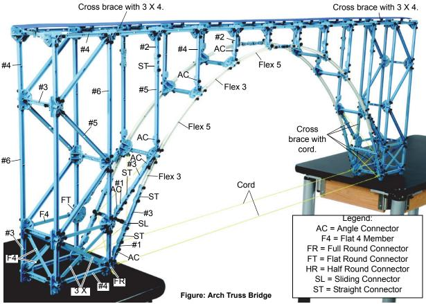
The Arch Truss design is one of the most frequently used designs in history. Construct the end supports and then add the deck. Tie cords from the base of one end support to the base of the other end support. Next, add the arch and suspension beams. Use Flat 3 X 4 members to cross brace the deck at the point where it joins the top of the end supports. Use cord to cross brace the bottom sections of the arch. Finally, use Track Clips to attach the Coaster Track.
