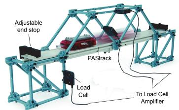
Recording the forces measured by the load cells as the cart traverses the PAStrack bridge.
