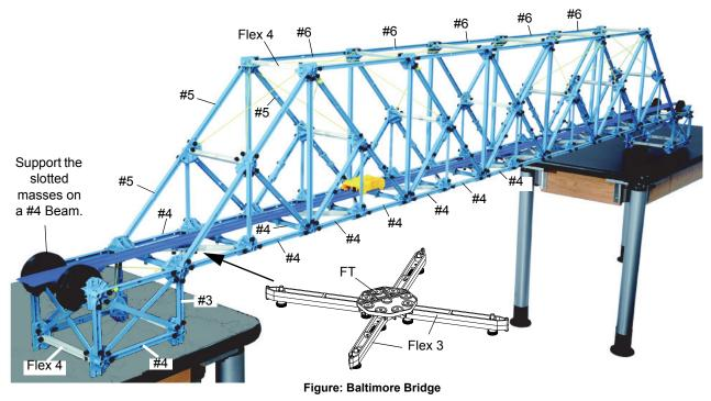
Use Flat Round Connectors and four Flexible #3 Beams to make four cross braces for the deck. Place one at each end of the deck where it joins the end support and put the other two on both sides of the center of the deck.
