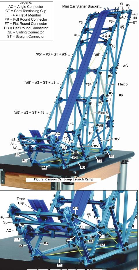
Figure: Canyon Car Jump Ramp Detail
