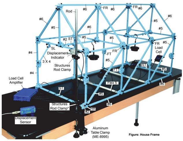
To hold the House Frame in place, attach a #2 Beam to the Half Round Connector at one corner. Put a clamp on the edge of the table and use it to hold a support rod (ME-8995). Attach a Structures Rod Clamp between the support rod and the #2 Beam at the corner of the House Frame.
