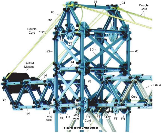
Put a Collet on each side of the Pulley to keep it in place on the front Long Axle. Make sure that the front Full Round Connectors are oriented so that the "fin" is vertical.
