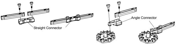
To use the sliding connector, loosen the thumbscrew and rotate the top "jaw" to the side. Place the beam onto the lower part of the connector, rotate the top "jaw" into place, and tighten the thumbscrew. The Structures Set includes two Angle Connector sets.
