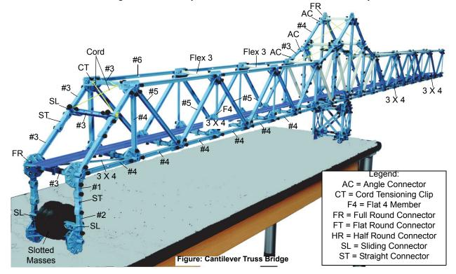
Use cord and Cross Tensioning Clips to cross brace the top section of the truss at the end of the bridge. Use Track Clips to attach the Coaster Track to the #3 Beam cross members. On each "arm" of the bridge, use a Flat 3 X 4 Member to cross brace the first section and the fifth section (counting from the end toward the tower).
