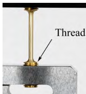
Figure 4: Center Threads in Load Cell
