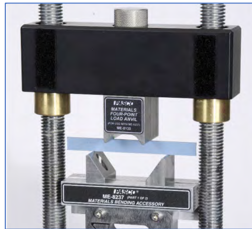
Figure 1: Four-Point Bending Test
