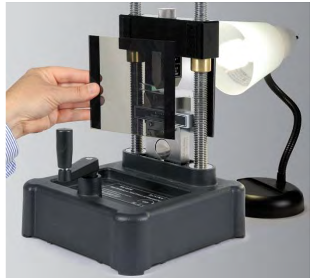
Figure 1: Viewing stress lines
