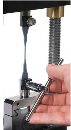
Figure 4: Tighten hex nuts
