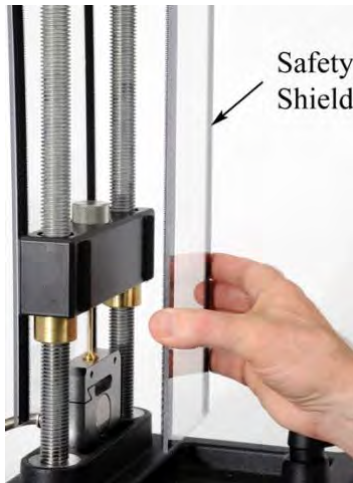
Figure 5: Always use Safety Shields!
