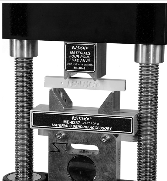
Figure 9: Testing a Cast Beam using the Bending Accessory and Four-Point Load Anvil.
