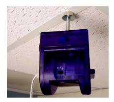
3. Rotate the sensor head to point downward.
