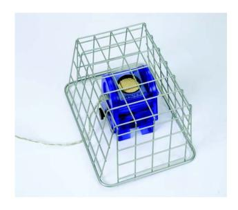
Position the guard so that the intersections of the wires are not directly above the sensing element.
