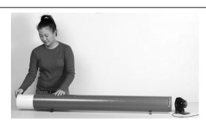
Figure 1: Placement of Resonance Tube relative to the Open Speaker
