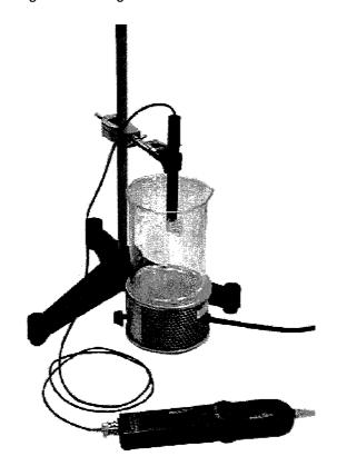
In addition, ORP studies are temperature-dependent. To ensure that temperature is accounted for, it is best to use a Temperature probe in the pH/ORP/ISE Amplifier's stereo plug.
