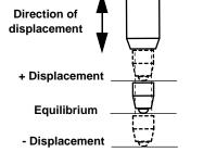
If the object will be displaced both positively and negatively from its equilibrium position, adjust the indicator so that the position of the measurement head when it is in contact with the object is about halfway between the limits of the measurement head's travel. Press and release the ON/O button to zero the indicator when the measurement head is at the equilibrium position.
