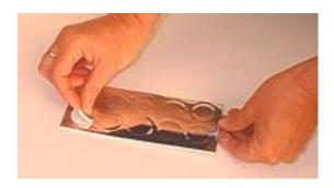
2. Carefully remove the protective backing paper.
