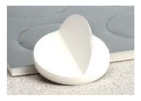
3. Place the Fast Response Temperature Probe
