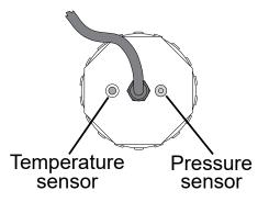
The depth sensor is a gauge-type pressure sensor with a stainless steel housing and a stainless steel diaphragm. The entire sensor head is designed to resist the corrosive effects of salt water.
