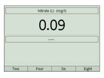
To remove the measurement from the lower segment of the Digits screen: Press . Press the down arrow to highlight the data source field of the lower segment. Press again to open the menu. Use the arrow keys to highlight Clear Input and press .
