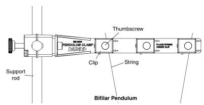
designed so that the string or thread is held under the edge that is the farthest from the rod clamp. Arrows next to each clip point the way. Tighten the thumbscrews to hold the string in place.
