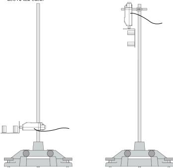
3. Insert the model rocket engine into the test stand with the engine's exhaust port pointing away from the force sensor.
