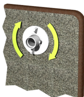
Figure 2: Tightening the nut on the insert.
