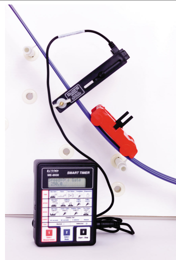
Figure 11: Car with photogate flag moving toward a Photogate Head (ME-9498A).
