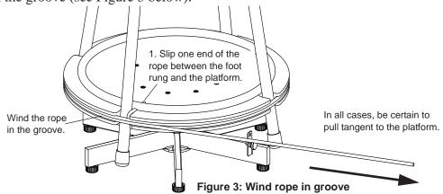
2. Be sure to pull the rope or cord free when finished applying the torque to the rotating chair.
