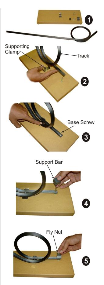
Picture - 5 Tighten Fly nut on supporting bar.
