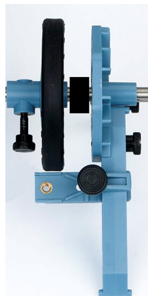
Figure 12: Sliding connector attached to I-beam.
