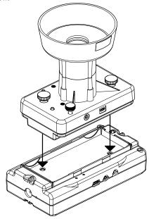
2. Turn each mounting thumbscrew until finger-tight to secure the accessory to the cart.
