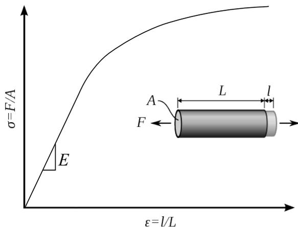
Figure 1: Stress-strain curve.
