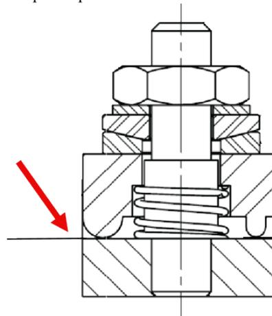
**NOTE:** The plastic test coupons have ridges on their top sides. Place the coupon end under the clamp top with the ridged side facing upwards.
