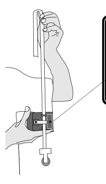
This timing method is a visual demonstration of speed and acceleration. A moving object pulls a paper tape through the timer which prints dots on the tape at even time intervals. The result is a series of dots in a line on the paper tape representing the position of the object as a function of time. From the dots on the tape, the distance traveled can be measured and the average speed for each time interval calculated.
