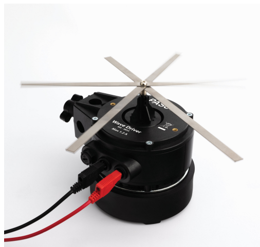
Figure 1. Proper setup for the Metal Resonance Strips on the Wave Driver (WA-9855).
