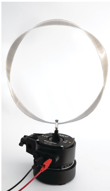
Figure 1. The proper experimental setup for using the Resonance Wire Loop in a vertical orientation.
