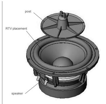
Figure 1. Alignment of Post on Speaker
