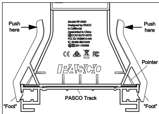
Slide the Light Source along the track to the desired position. Note that there is a pointer on both sides of the Light Source that will indicate the position of the central RGB LED for measurement purposes.
