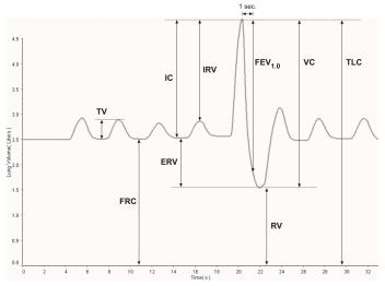
When performed correctly, a plot of lung volume versus time for the experiment described in **Data collection** will yield data similar to what is shown above. The following values can be obtained from such a plot:
